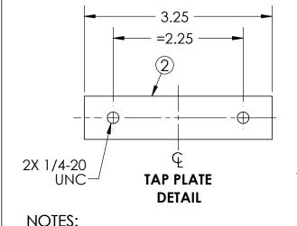
. MATERIALS AND FINISHES: WELDED STRIKER PIN, TAP PLATE AND BRACKET TO BE OF 1018 COLD ROLLED STEEL. ALL COMPONENTS TO BE CLEAR ZINC PLATED
