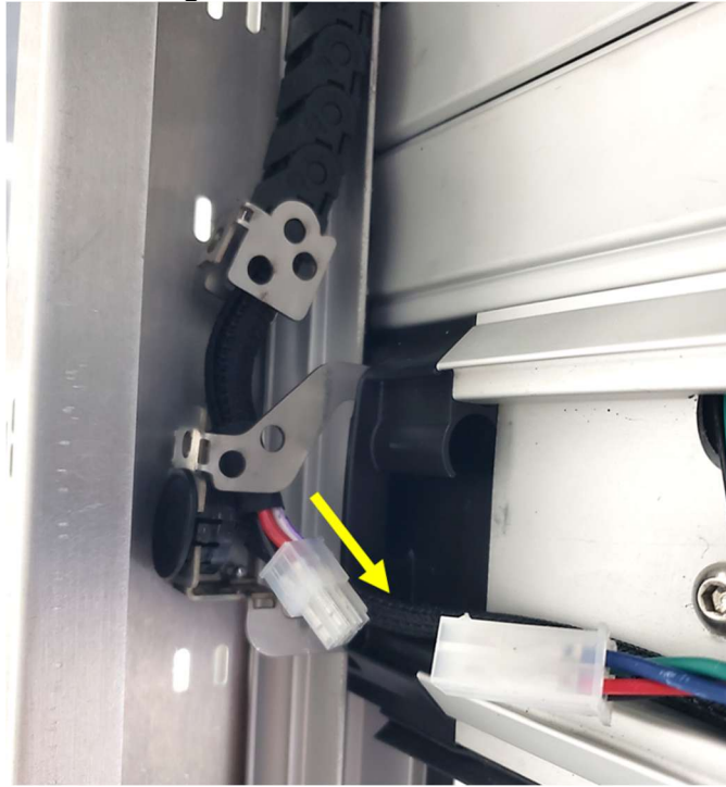
Figure 35. Route the cable through the sensor bracket
